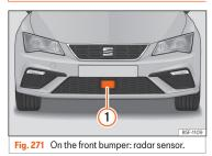
A radar sensor is installed on the front bumper to determine the traffic situation **>>> Fig. 271** (1).
