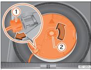
Fig. 318 In the boot: remove the subwoofer.
