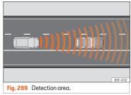
The adaptive cruise control (ACC) is an extension of the normal cruise control system (CCS)  $\cdots$   $\Delta$ .
