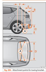
If a towing bracket is to be fitted after the vehicle is purchased, this must be completed according to the instructions of the towing bracket manufacturer. The attachment points for the towing bracket (A) are on the lower part of the vehicle.
