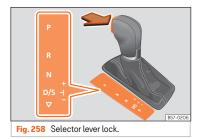
The selector lever lock prevents gears from being engaged inadvertently, so that the vehicle is not set in motion unintentionally.
