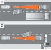
**Fig. 276** (C) Vehicle changing lanes. (D) One vehicle turning and another stationary.
