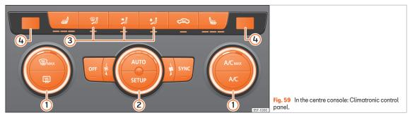
To switch a specific function on, press the appropriate button. Press the button again to switch off the function.
