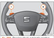
Fig. 260 Steering wheel: automatic gearbox levers
