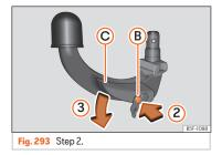
Before assembling it, place the detachable ball in the standby position with the following two steps.
