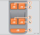
**Fig. 14** Detail of the driver door: controls for the windows.
