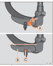
Fig. 294 Reserve position: position of the lever and the release bolt.
