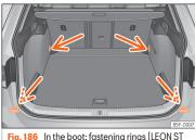
Fig. 186 In the boot: fastening rings (LEON ST model).
