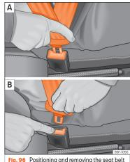
Fig. 96 Positioning and removing the seat bel buckle.
