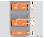
**Fig. 148** Detail of the driver door: controls for the windows.
