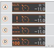
Fig. 264 Instrument panel display: CCS status indications.
