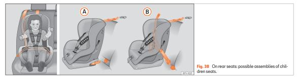
Figure **>>>** Fig. 38 (a) shows the basic child restraint system mounting using lower retaining rings and the upper retaining strap. Figure **>>>** Fig. 38 (b) shows the child restraint system mounting using the vehicle seat belt.
