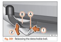
Do not omit this first step **>>> page 304, Re**moving the tow hitch. Step 1!
