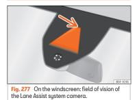
Using the camera located in the windscreen, the Lane Assist system detects the possible lines dividing the lanes. When the vehicle involuntarily approaches a dividing line it has detected, the system notifies the driver with a *corrective steering movement*. The purpose is not only to warn the driver, but also to keep the vehicle inside the lane. This movement can be over-regulated at any time.
