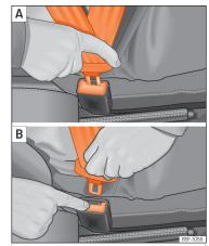
Fig. 21 Positioning and removing the seat belt buckle.
