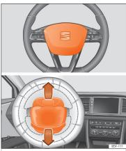
Fig. 26 Driver airbag located in steering wheel.
