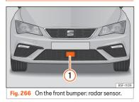
A radar sensor is installed on the front bumper to determine the traffic situation **\*\*\* Fig. 266 (1)**. The radar sensor's visibility may be impaired by dirt, mud or snow, or by environmental influences such as rain or mist. In this case, the Front Assist does not work. The instrument panel displays the following message: **Front** Assist: No sensor vision! If necessary clean the radar sensor »» **0**.
