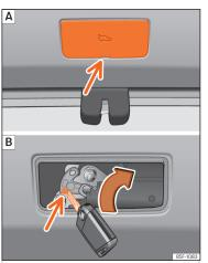
Fig. 10 Luggage compartment: access to manual release.
