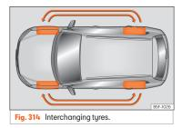
To ensure that the wear is equal on all tyres the wheels should be changed round from time to time according to the system  $\mathbf{w}$  Fig. 314. The useful life of all the tyres will then be about the same time.
