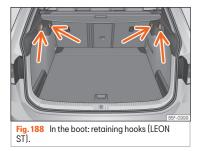
At the rear of the luggage compartment, on the left and right, there are fixed retaining hooks **>>> Fig. 188**.
