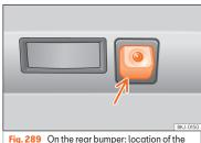
**Fig. 289** On the rear bumper: location of the rear assist camera.
