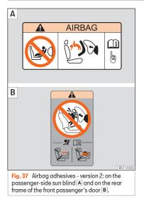
A sticker with important information about the passenger airbag is located on the passenger's sun visor and/or on the passenger side door frame.
